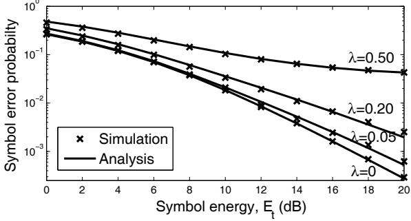
Fig. 2. SEP as a function of  $E_t$  for different values of  $\lambda$ , each of which corresponds to a different value of  $\frac{I_{\text{ave}}}{E_t}$  (QPSK).
