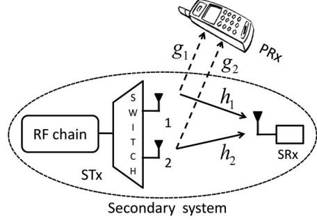
Fig. 1. System model with one PRx and a secondary system consisting of a STx with two transmit antennas and one RF chain that communicates with a SRx with one receive antenna.
