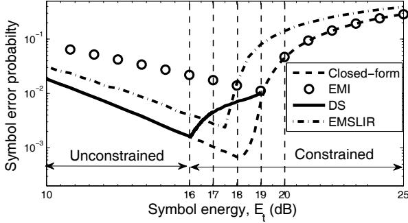
Fig. 4. Comparison of the SEPs of the closed-form optimal AS rule and several benchmark rules ( $I_{\text{ave}} = 16$  dB and QPSK).
