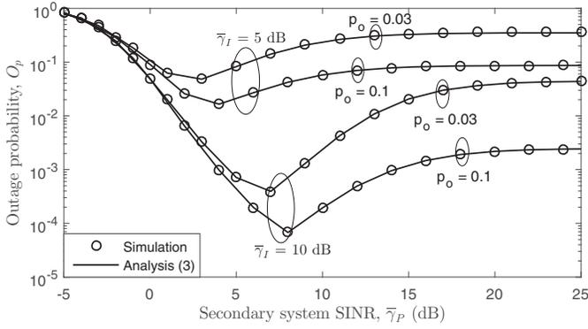
Fig. 2. Outage probability versus secondary system SINR for different values of  $\bar{\gamma}_I$  and  $p_o$  ( $P_p/\sigma^2 = 5$  dB,  $N_S = 3$ ,  $N_D = 4$ , and  $L = 3$ ).
