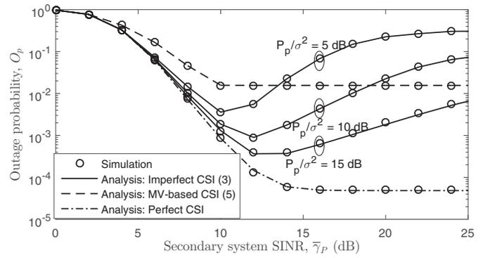
Fig. 4. Impact of different CSI availability ( $r = 2$  bps/Hz,  $p_o = 0.01$ ,  $\bar{\gamma}_I = 15$  dB,  $N_S = 4$ ,  $N_D = 5$ , and  $L = 3$ ).
