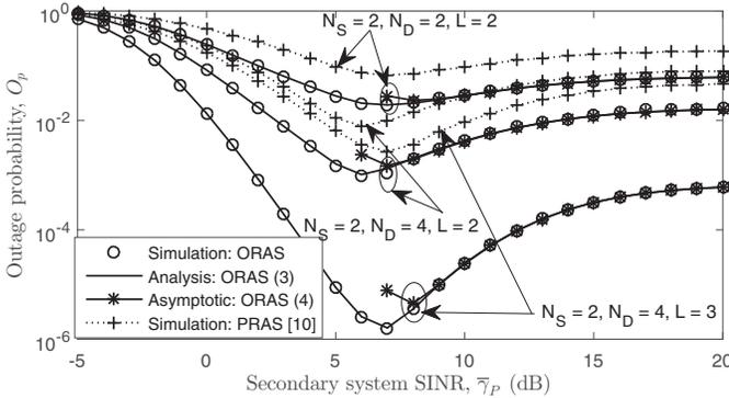
Fig. 3. Outage probability versus secondary system SINR for different number of antennas and relays ( $P_p/\sigma^2 = 5$  dB,  $p_o = 0.1$ ,  $\bar{\gamma}_I = 8$  dB).
