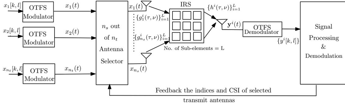
Fig. 1: System Model for Multiple Input Single Output IRS-Aided OTFS under Transmit AS
