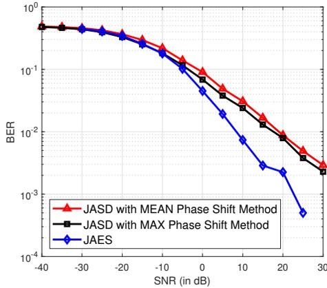
Fig. 3: BER performance for a ( $n_t = 4$ ,  $n_s = 2$ ,  $L = 6$ ) IRS-aided OTFS system with the proposed algorithms
