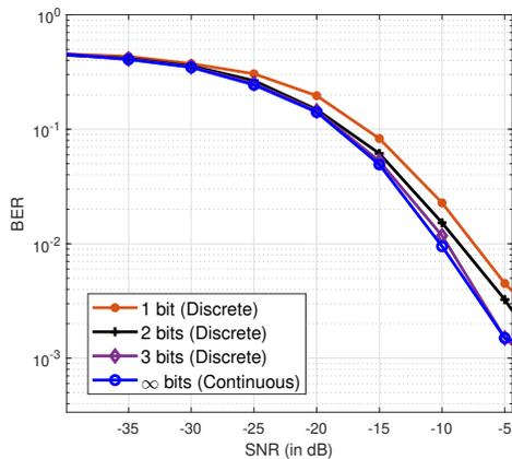
Fig. 4: JAES: Impact of discrete phase shifts on BER ( $n_t = 4$ ,  $n_s = 2$ ,  $L = 24$ ,  $U = 10^4$ )
